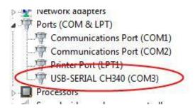
6. Open the computer software as shown in the figure below, and pay attention to selecting the corresponding "port". The "communication baud rate" and "slave address" should be consistent with the internal settings of the DPM8600 power supply. The default communication baud rate of the machine is "9600" and the slave address is "1"; then click the "connect", the model and serial number displayed, indicating that the connection is finished.
