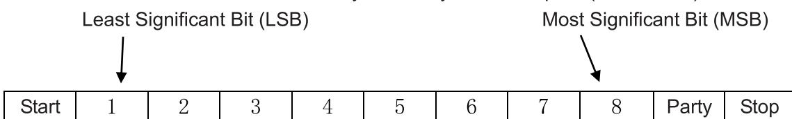
Transmit Character = Start Bit + Data Byte + 2 Stop Bits (11 bits total):
